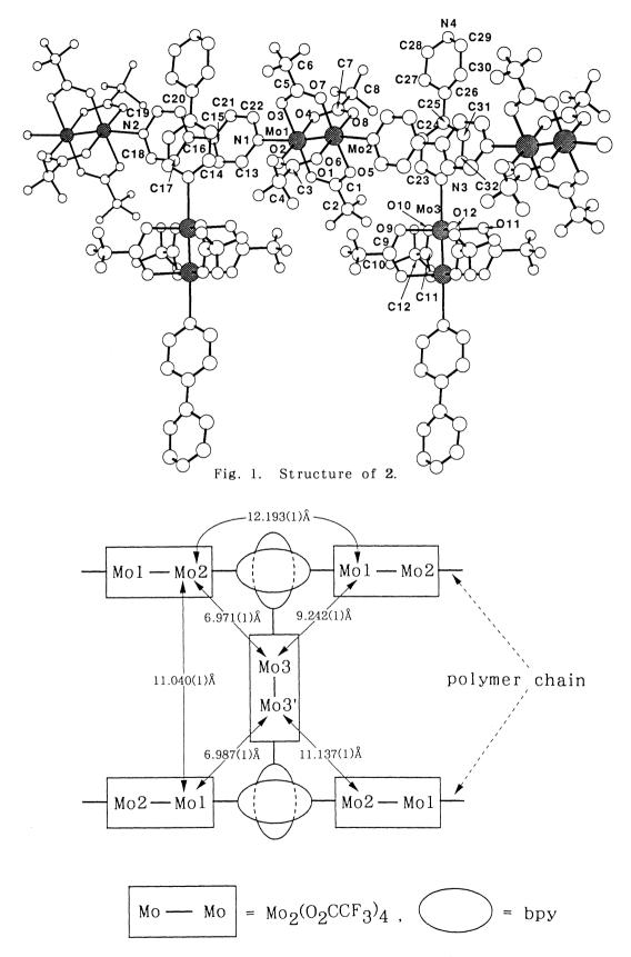
Fig. 2. Correlation between the  $\mathrm{Mo_2(O_2CCF_3)_4}$  cores.
